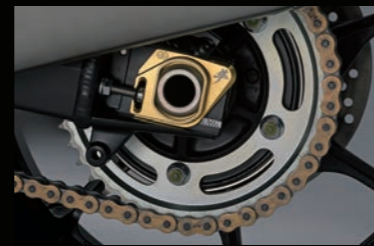
Aluminum chain adjuster 99117-10L00-000 Aluminum chain adjuster with Hayabusa logo. *Set of right and left side.
