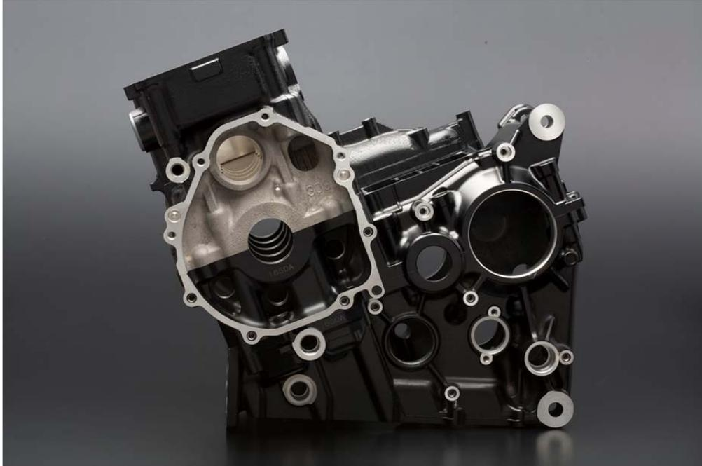
Ventilation holes are added to the bottom side of each cylinder located on the “cylinder integrated 3-piece crankcase”. These ventilation holes reduce pumping loss.
